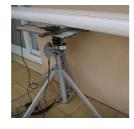
4 telescoping legs for unneven ground and Operation in confined space. Special design to work close to the wall
